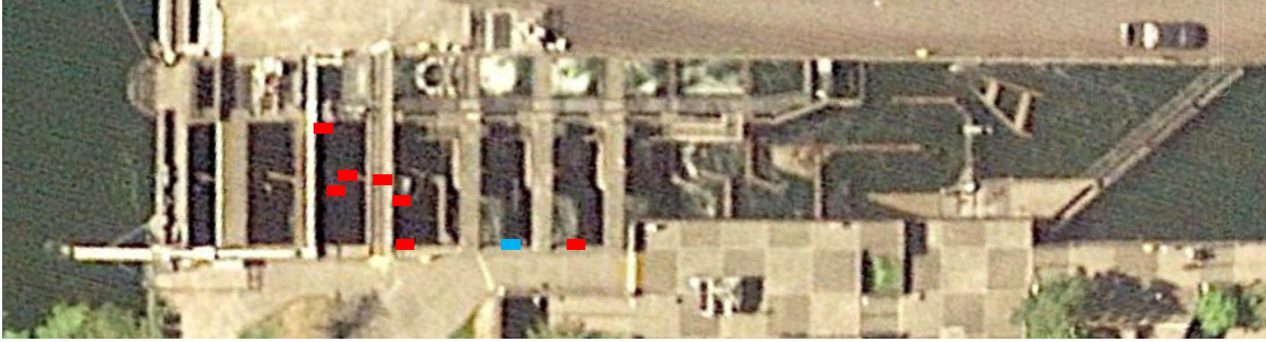
Figure 2. Overview of “puck” placement areas on aerial photo. The red lines represent 4 inch pucks and the blue lines represent 8 inch pucks.
